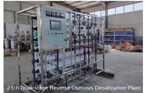
2 t/h Dual-stage Reverse Osmosis Desalination Plant
