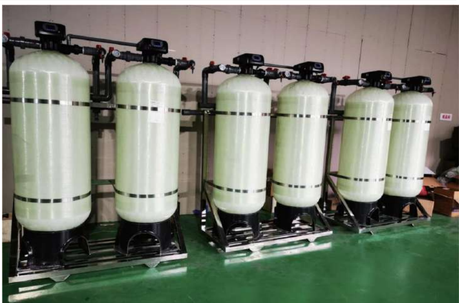
Boiler Water Softening Equipment
