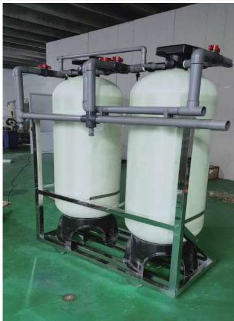
Boiler Water Softening Equipment
